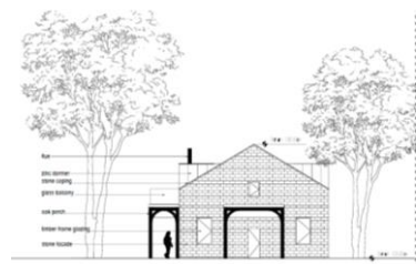
North-east elevation (facing rear of the site)
