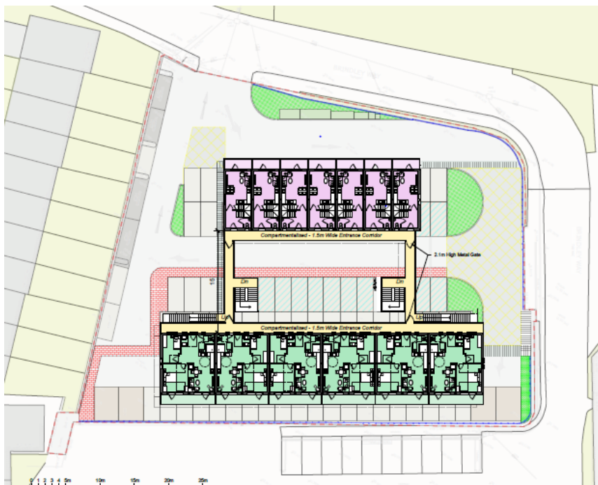
Fig 3: Proposed first floor plan (Terrace A colour in purple and Terrace B colour in green)
