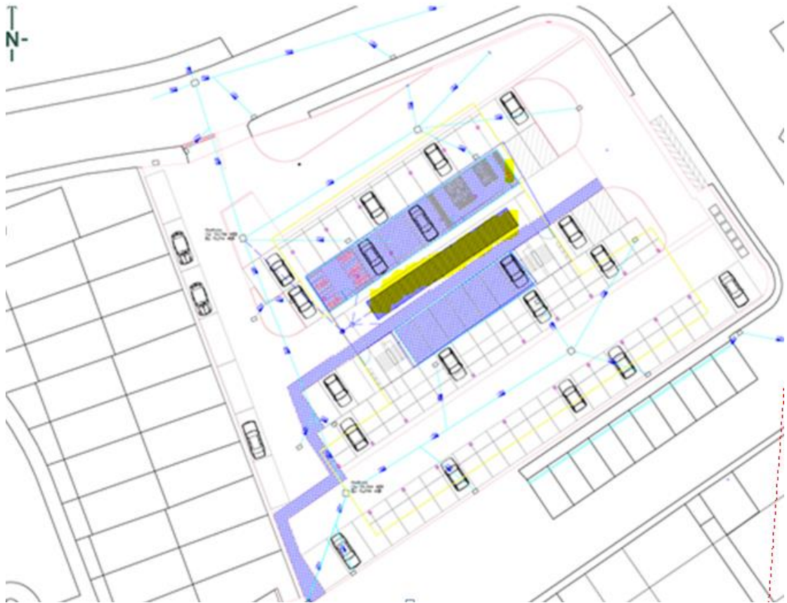
Fig 13. Location of porous paving and underground attenuation tank. (Porous paving colour in blue. Underground attenuation tank colour in yellow)
